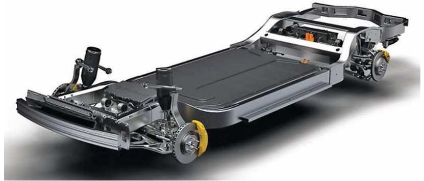
Fig. 5. The skateboard chassis for EVs can be used for various vehicles. (Image courtesy Rivian.)
