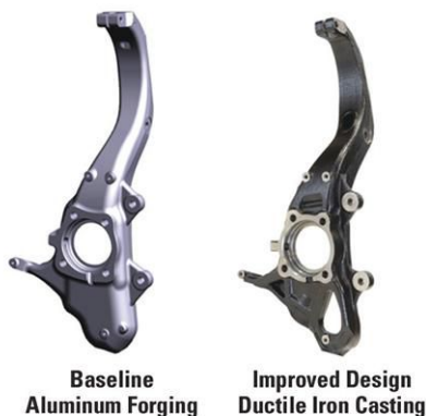
Fig. 1. The steering knuckle conversion from an aluminum forging to a ductile iron casting achieved a 40% cost savings and 30% reduction in weight, while improving strength and stiffness by 20% and 25%. (Photo courtesy of Waupaca Foundry)
