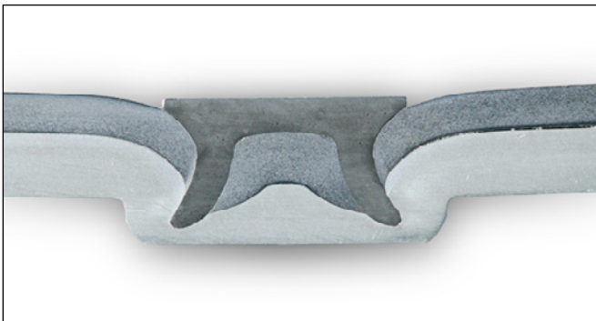
Figure 3. The Tucker® self-piercing rivet is capable of joining aluminum to steel. (Source: Stanley Engineered Fastening.)
