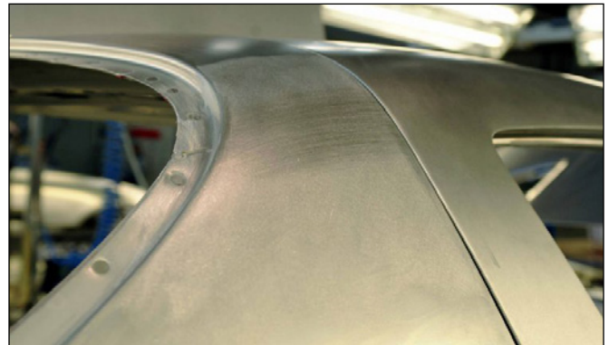
Figure 1. An aluminum component welded by Magna using the CMT technology developed by Fronius. (Source: Fronius.)
