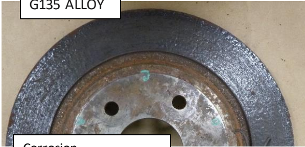
Corrosion Scale on Brake Surface
